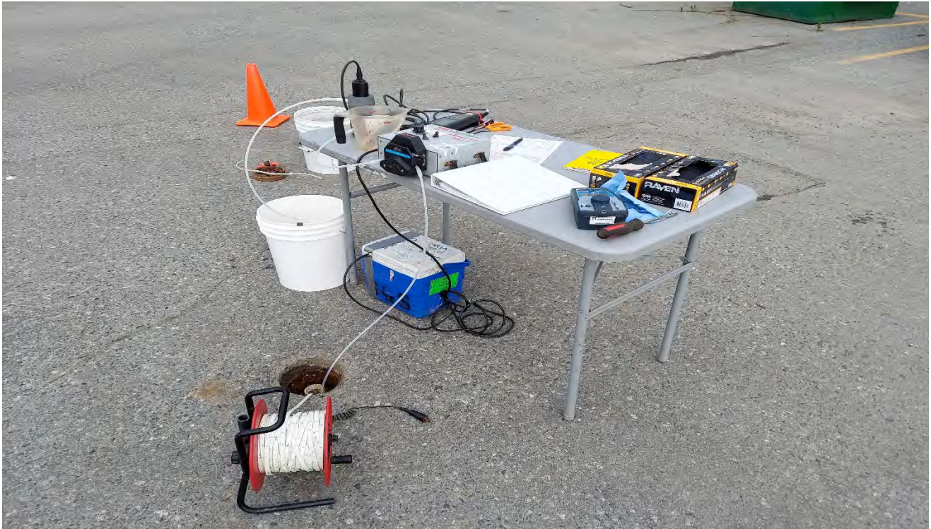
Photo 5: Purging well C-1. (7/14/21)
