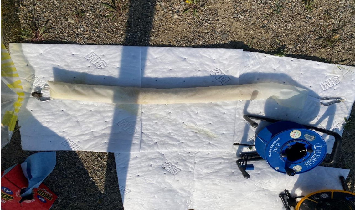
Photo 3: Sorbent sock used to absorb product from MW-5 (June 27, 2024)
