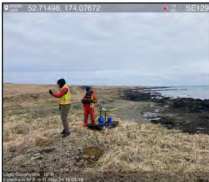
Photo 1: The 200-MHZ GPR system on Eareckson in the sled used for acquisition. Note the sled puller, on the right, referencing his mobile device for positioning.
