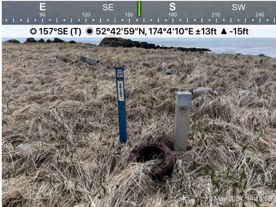
Photograph 03: LF024 groundwater monitoring well SW10W2 and metal surface debris.
