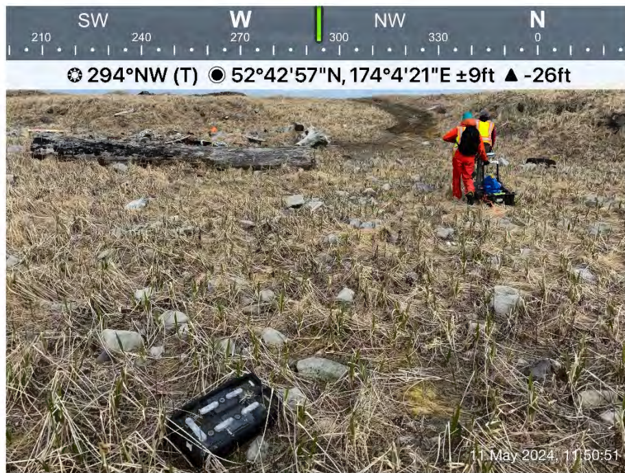
Photograph 16: LF024 GPR survey in progress and an intact lead acid battery near the end of the access road in the spray zone.
