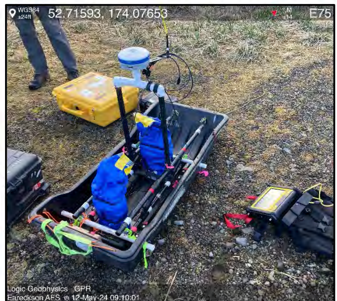
Photo 2: The 200-MHZ GPR system on Eareckson in the sled used for acquisition. The controller is on the ground on the right.
