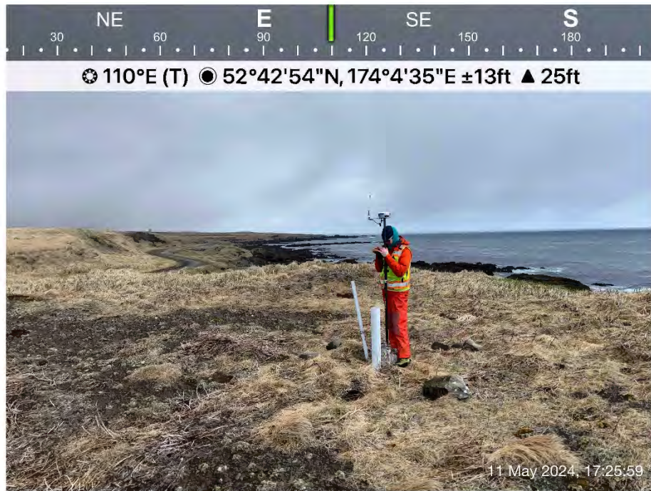
Photograph 38: Daily GPS check shot location at LF026 cut off telephone pole control point.
