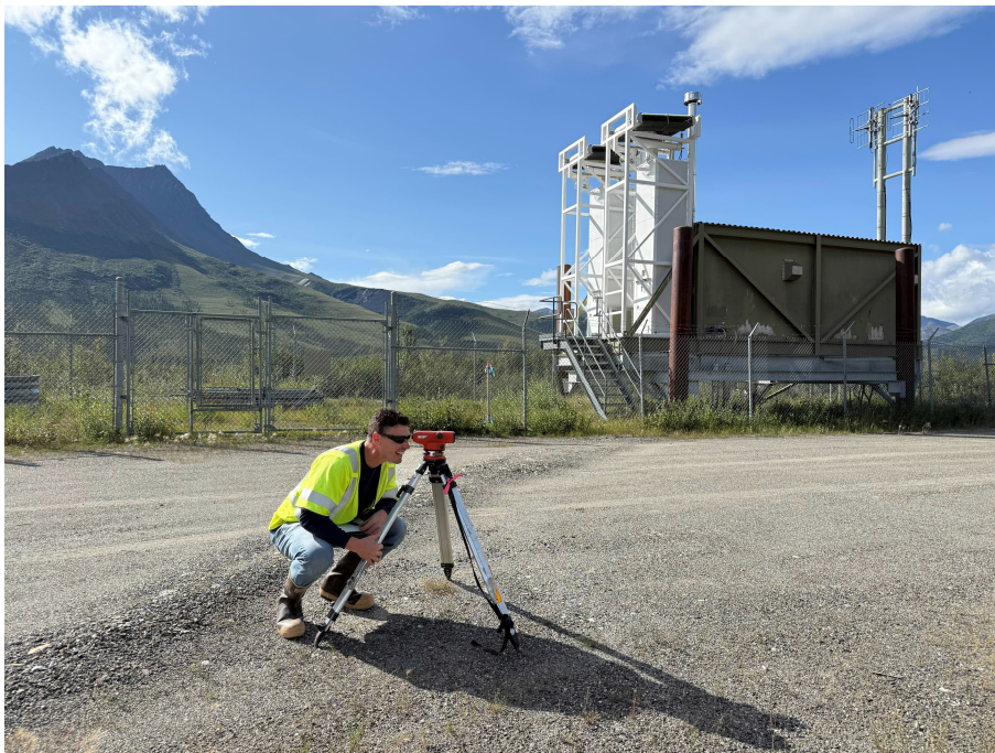
Photo 2: Performing a level loop survey (August 5, 2025)
