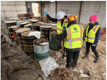
Making visual observations of liquid drum contents using a drum thief. View looking SW. (16OCT2025)
