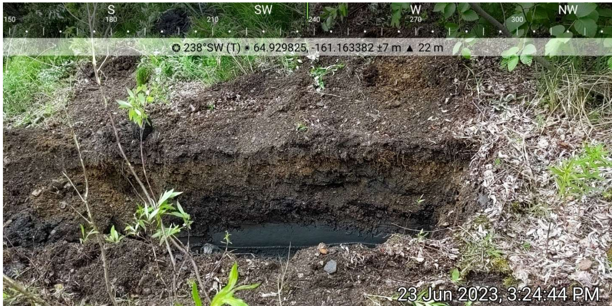
Photo 11. Test pit TP6. The upper two feet of the profile is coarse-grained fill material, while silt-rich native soil is present below a depth of two feet. June 23, 2023.
