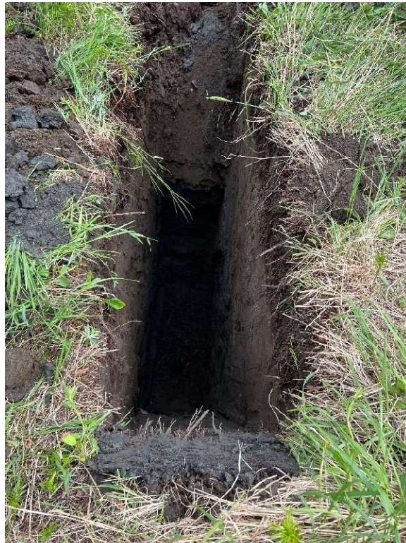
Photo 2. Test pit TP1. Native topsoil is visible over grayish silt. June 22, 2023.
