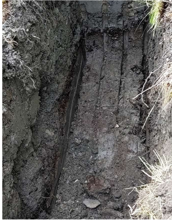
Photo 5. Test Pit TP2. Soil staining and petroleum product are visible. June 22, 2023.
