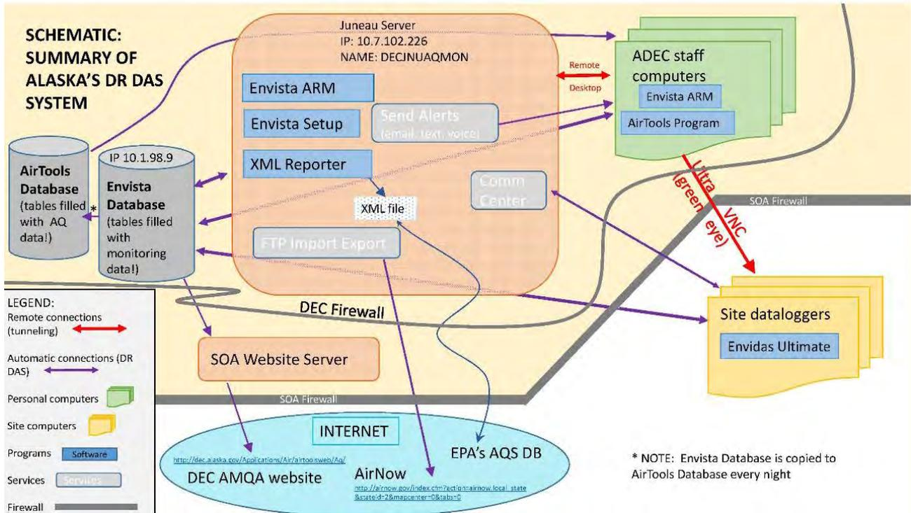
Figure 15. Schematic of Alaska's DAS
