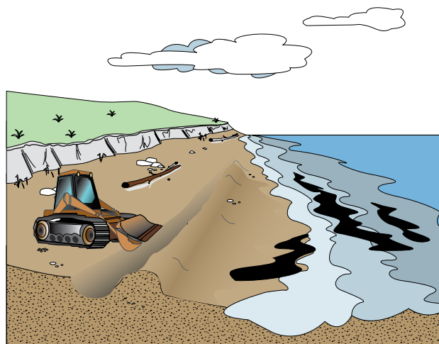
Figure BB-1. Beach berm construction.
