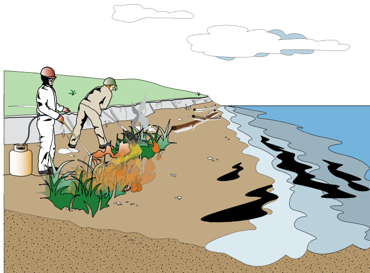
Figure ISv-2. In-situ burning on beach environment.
