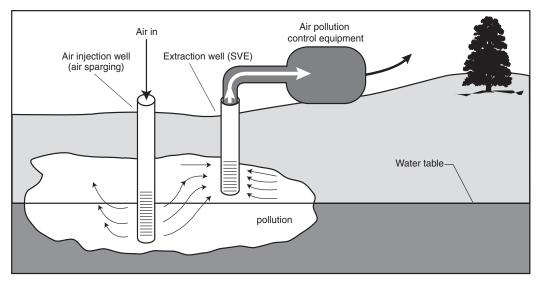
The air used in SVE and air sparging also helps clean up pollution by encouraging the growth of *microbes*. These tiny bugs are found naturally in soil and can use pollution for food. When microbes completely digest pollution, they can change it into water and harmless vapors. (*A Citizen's Guide to Bioremediation* [EPA 542-F-01-001] describes how microbes work.)
