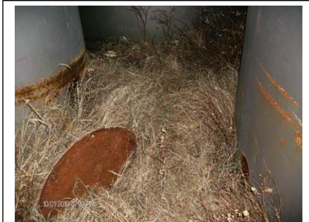
Photograph 5.2-2: ASTs stored at the Barge Landing Area, showing holes cut in tanks and a removed cover. These tanks are thought to be from the Former AVEC Facility. (10/1/2010)
