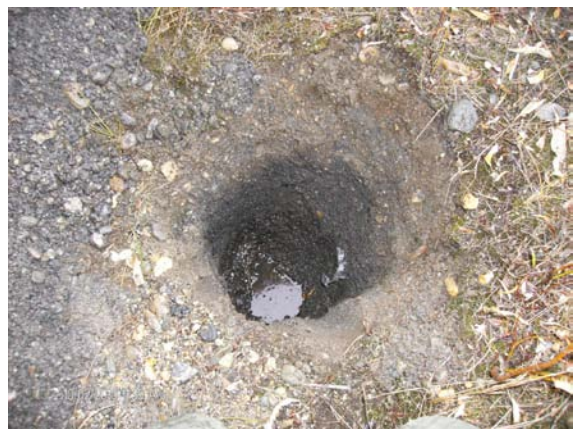
Photograph 7.2-6: Former School Tank Farm Test Pit SF1 with staining, oily water entry at the base, and polyethylene sheeting visible in the right hand side of the test pit. (10/2/2010)
