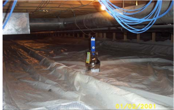
Crawl space samples are collected in a similar manner to indoor air. The canister is simply placed in the space and opened.
