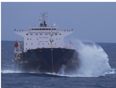
The Golden Seas in tow with the ADEC Emergency Towing System. (Photo courtesy of USCG)
