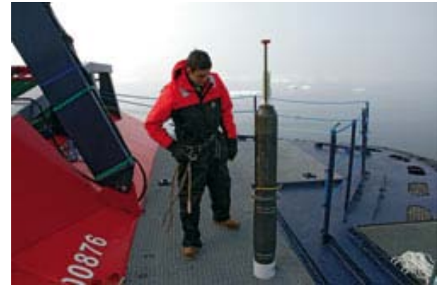
Luc Rainville, on the Swedish icebreaker Oden in August 2005, prepares to test an experimental float designed for under-ice operations in the Arctic. (Photo by P. Winsor)
