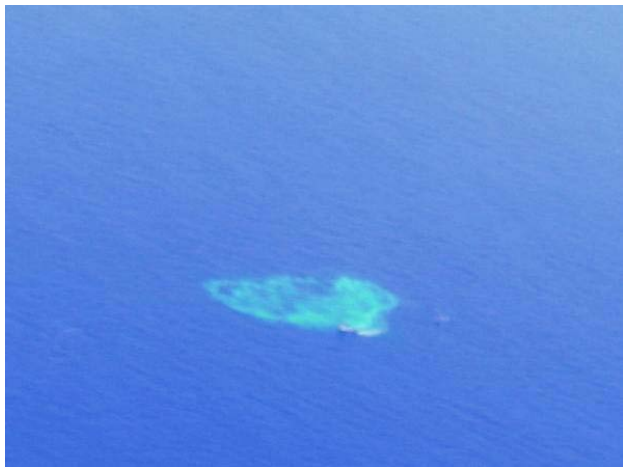
SIO 2005 – dye dispersion experiment using CTD, drifters and fluorometer
