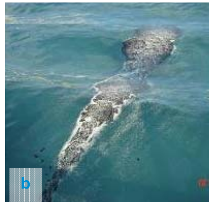
California OCS crude oil after application of a) COREXIT 9500 and b) dispersant gel.
