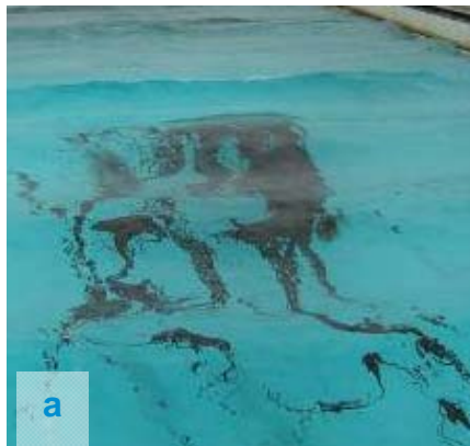
California OCS crude oil after application of a) COREXIT 9500 and b) dispersant gel.
