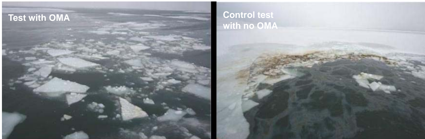
Photos taken during field tests of OMA-treated oil in ice after enhancing the dispersion with propeller wash of an icebreaker
