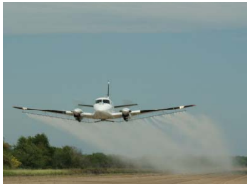
Gel dispersant effectively sprayed from an airplane
