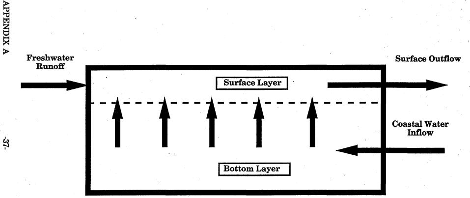
Figure 11. Schematic diagram of estuarine flow in Akutan Harbor during Summer season when stratification is present.
