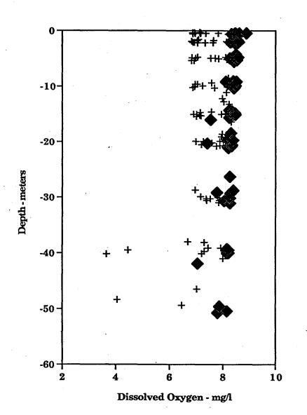
Figure 1. Dissolved oxygen in Akutan Harbor using data collected September 3, 1993.
