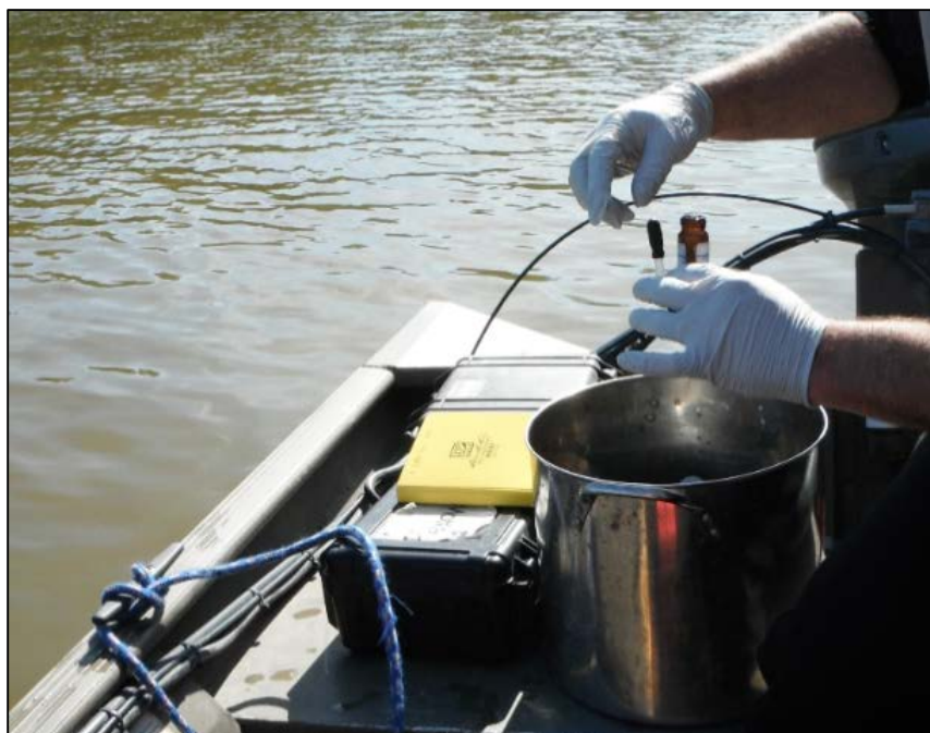
Process of collecting a TAH sample. The vials are preserved with hydrochloric acid, kept in a cooler at less than 6 degrees Celsius and then shipped to the laboratory for analysis.
