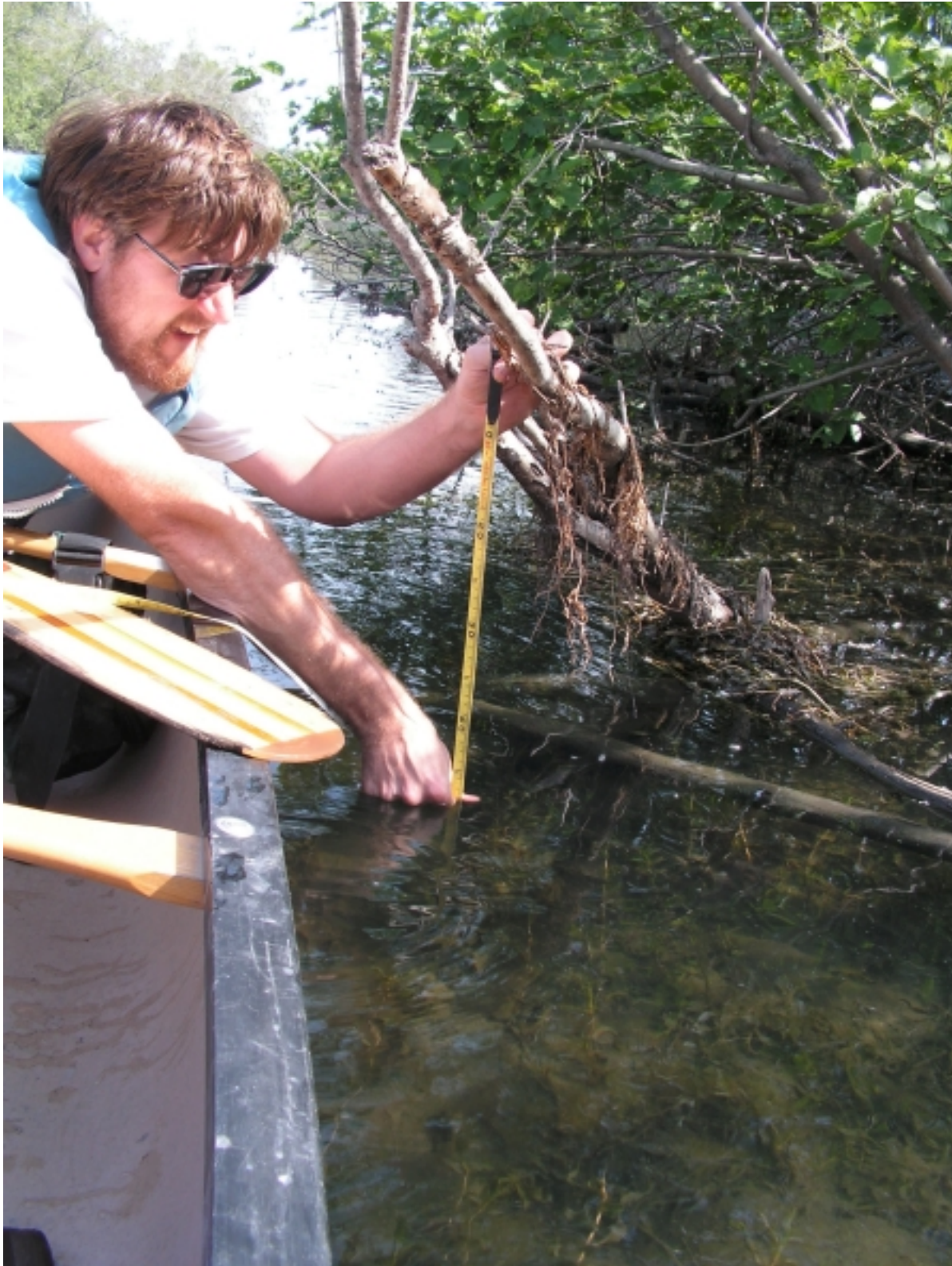
Figure 57. Aquatic vegetation suspended from branches after watercraft passed along Jim Creek, Alaska, demonstrating that boat wakes exceeded 40cm, 2009.
