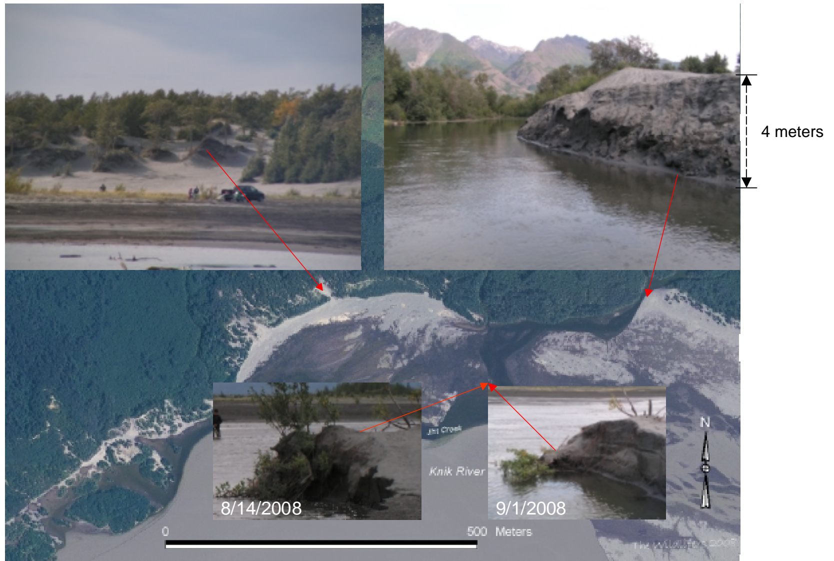
Figure 53. Example 2008 photos and locations of severe bank erosion and vegetation loss along Jim Creek Flats, Alaska.
