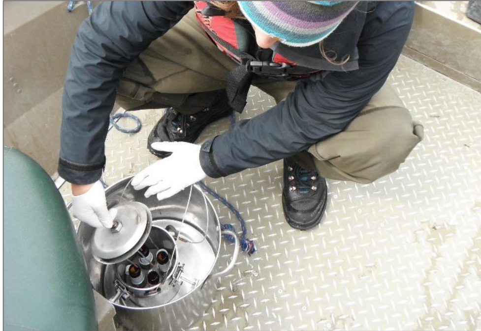
Photograph A11. Removing sample bottles from VOC sampler (8/3/14).
