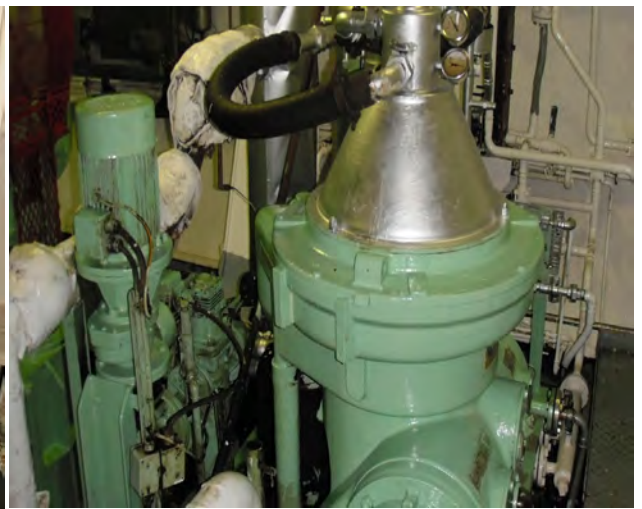
Photo 57: OWS separator/sludge treatment (dynamic) "concentrator"
