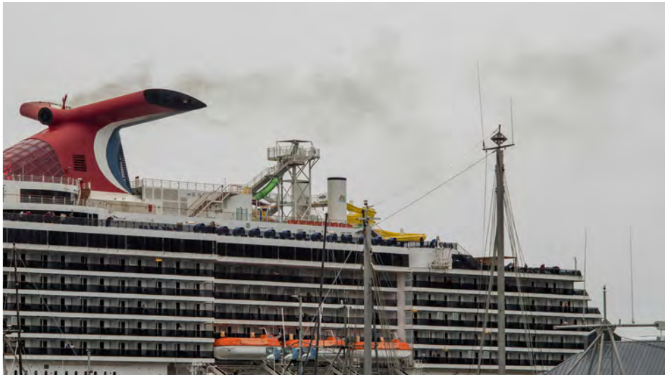
Photo 39: Black smoke caused by failure of fuel controller
