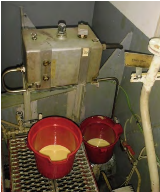
Photo 9: Example of leak potential into bilge
