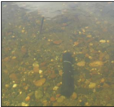
Water data logger is inside PVC housing and secured by cable to rebar.
