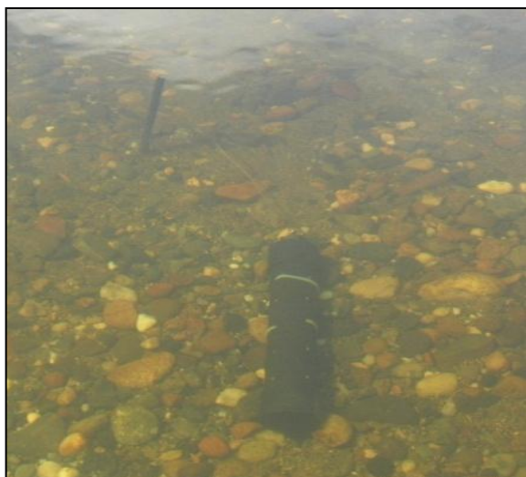
Water data logger is inside PVC housing and secured by cable to rebar.
