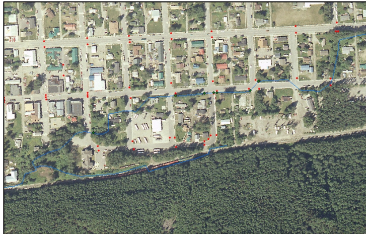
Catch basins are indicated in red in the example map above, Pullen Creek is shown in blue.
