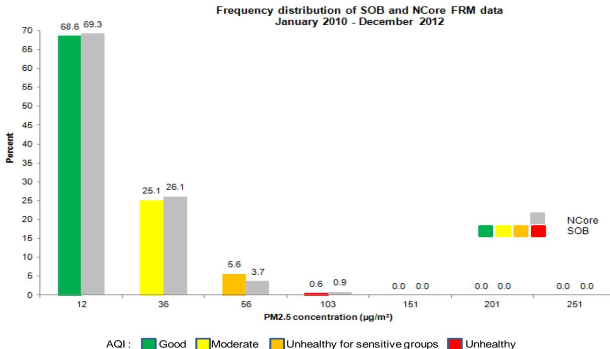
Figure 5-1. Frequency distribution of PM<sub>2.5</sub> concentrations for the Fairbanks SOB and NCore sites from January 2010 through December 2012
