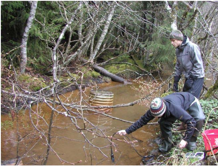
Figure 10. Sampling at site DC-A in April, 2006. The thick coating of iron floc on the streambed is easily disturbed by any activity (including sampling) in the stream. Caution is taken to avoid introducing re-suspended floc into the turbidity and TSS sample bottles, but this is not always possible.
