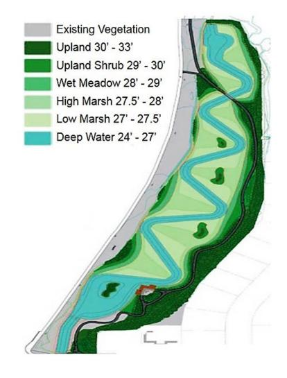
Figure 4. The Nancy Street Wetland design and plant list. Figure modified from Wright and Czapla (nd).
