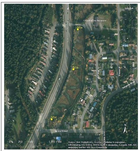
Figure 5. The Nancy Street wetland monitoring stations. The wetland inlet, NSa, is the upstream site where water flows into the wetland through a culvert under the Church od the Nazarene driveway. Site NSd is a midstream point within the wetland. Site NSd is just upstream of the wetland outlet, where the creek flows out of the wetland through two culverts under Nancy Street.
