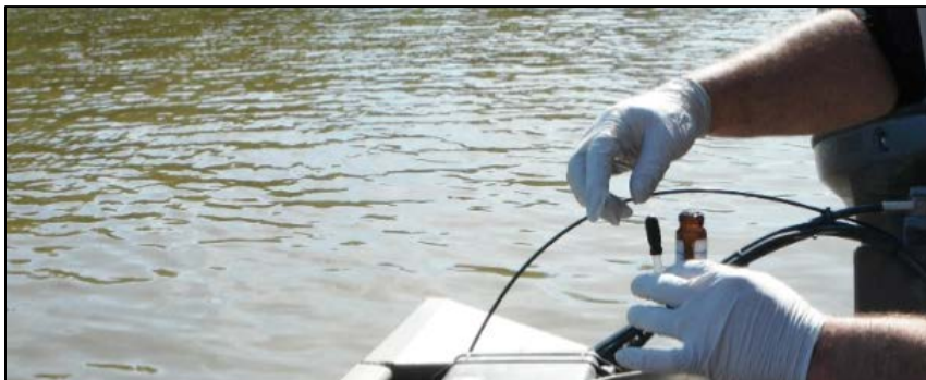
Process of collecting a TAH sample. The vials are preserved with hydrochloric acid, kept in a cooler at less than 6 degrees Celsius and then shipped to the laboratory for analysis.
