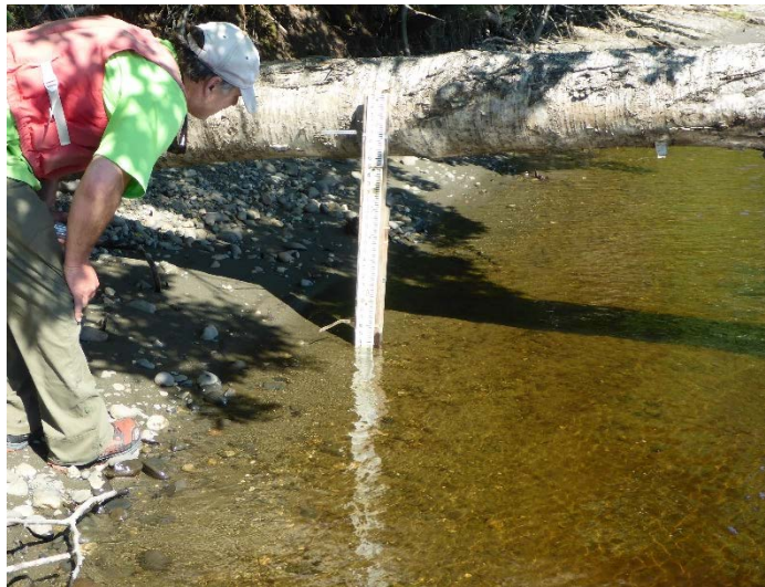
Photograph A4. Staff gauge and pressure logger at DR 0.75 (7/20/18).
