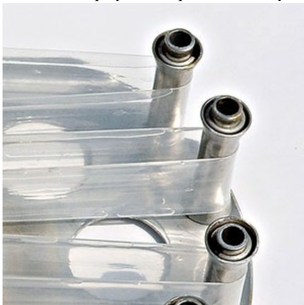
Figure 28. SPMD wound on sampling apparatus; source EST Labs, Inc.
