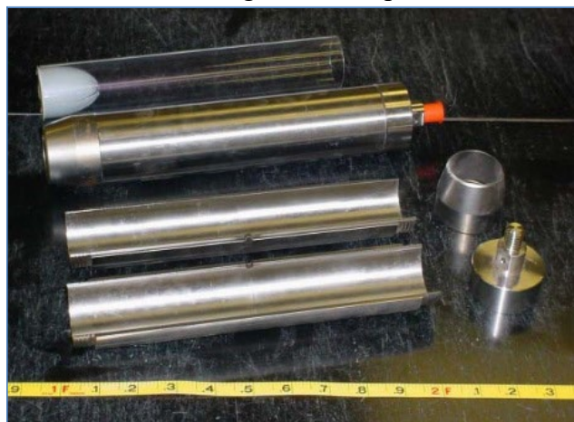
Figure 3. Soil Coring Device (Photograph by J. Schoenleber)
