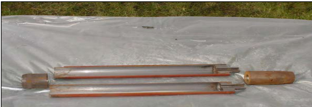
Figure 4. Split Spoon Sampler (Photograph by D. Dibblee)
