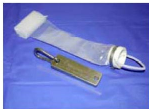
Figure 15. 1.5-inch Hydra Sleeve™ and stainless steel weight (1 liter capacity)
