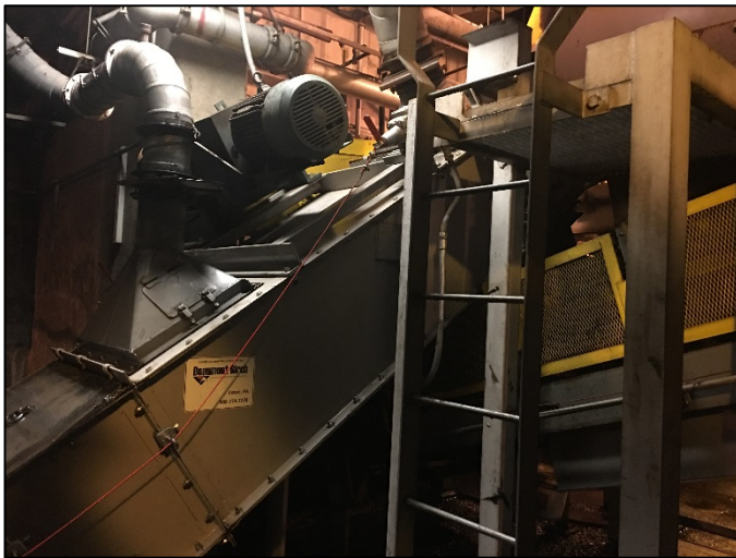
Coal Dust Control Suction in Enclosed Coal Conveyor
