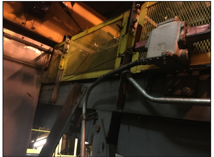
Enclosed Coal Conveyor from Coal Unloading to Coal Elevator
