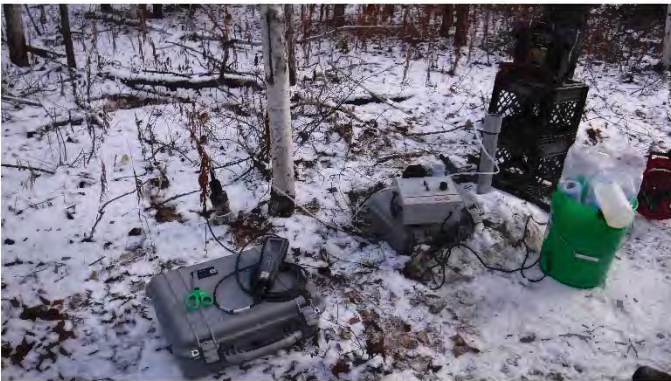
Photo 2: Sampling the unused well at 3485 Holden Road using a peristaltic pump. (October 23, 2017)
