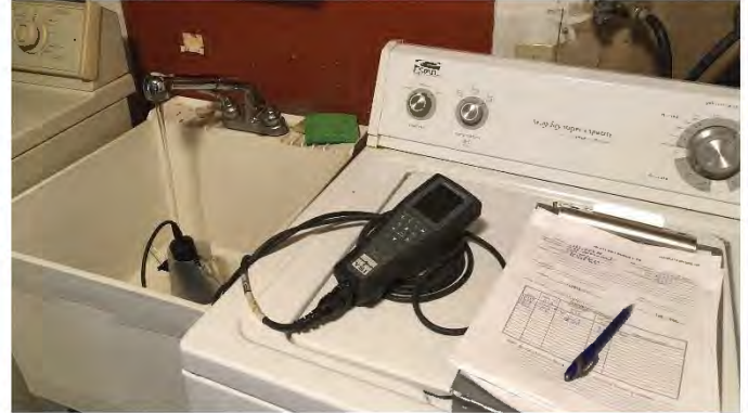
Photo 3: Example private well purge using YSI water quality meter, utility sink at 3077 Davis Road. (July 18, 2017)
