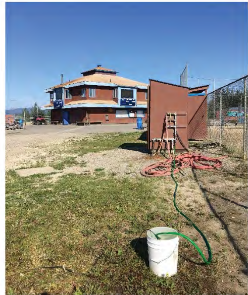
Photo 4: Purging the GHSA drinking water and irrigation well at the Hez-Ray sports complex to the ground surface before sampling. (July 19, 2017)
