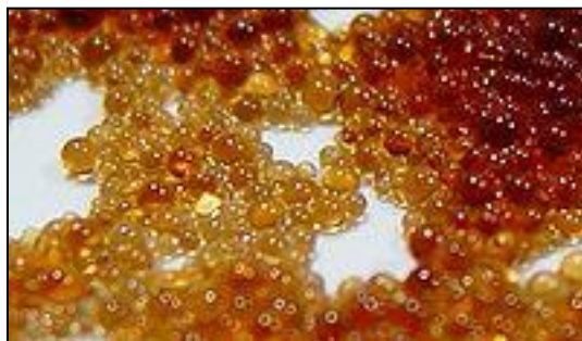
FIGURE 6 ION EXCHANGE RESIN BEADS [BIOTEC ENGINEERING]
