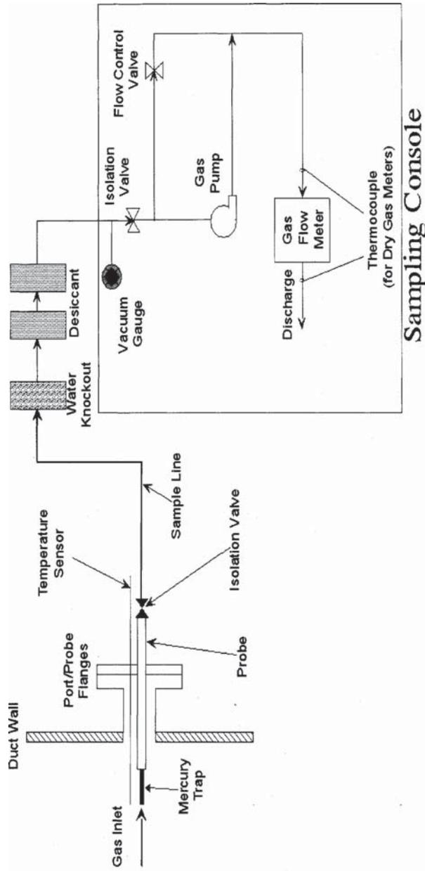
Figure 30B-1. Typical Sorbent Trap Sampling System
