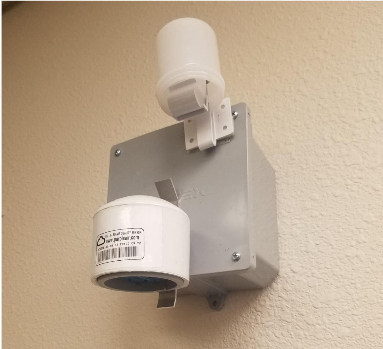
**Figure 4. PurpleAir unit and Ogawa SO<sub>2</sub> passive sampler attached to the junction box housing.**
