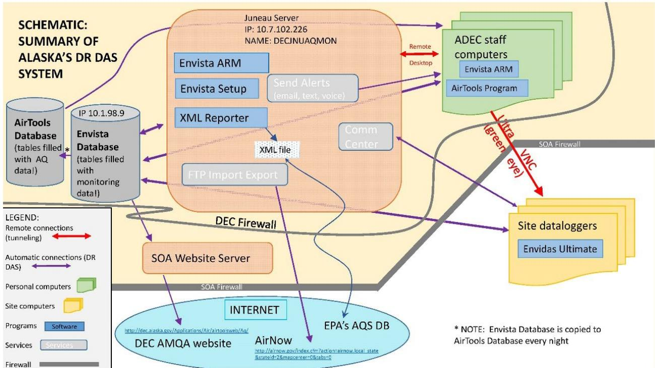
Figure 12. Schematic of Alaska's DAS
