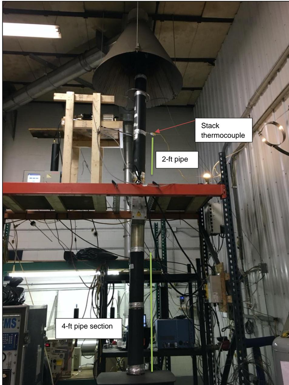
Figure 5. ESP installed on Cordwood Stove
