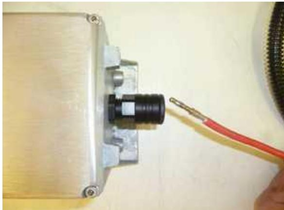
**CAUTION: When installing the high voltage cable, small loops and kinks in the cable must be avoided!**
