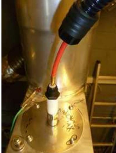
4. The high voltage cable must be fastened properly.
