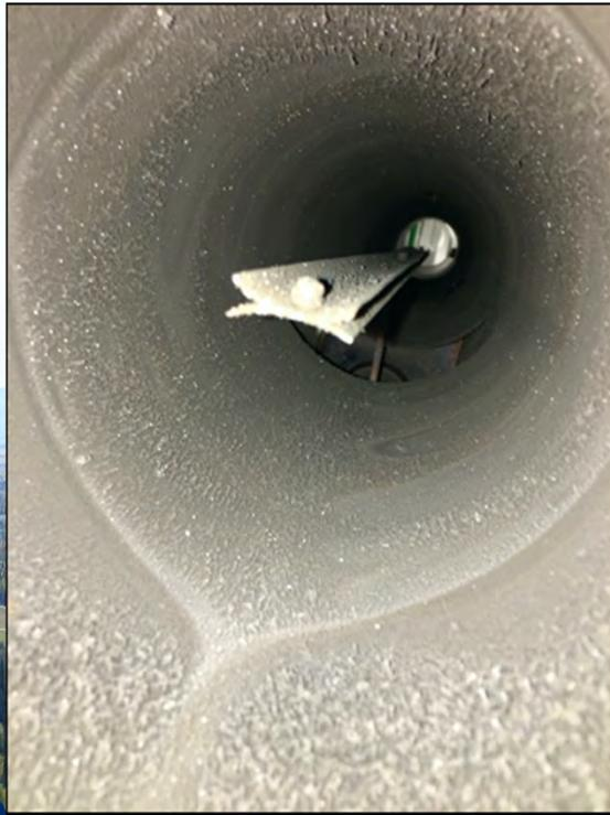
Creosote buildup after 34 hours of operation (after Run 3) on a non-catalytic cordwood appliance with dry fuel in a controlled environment
