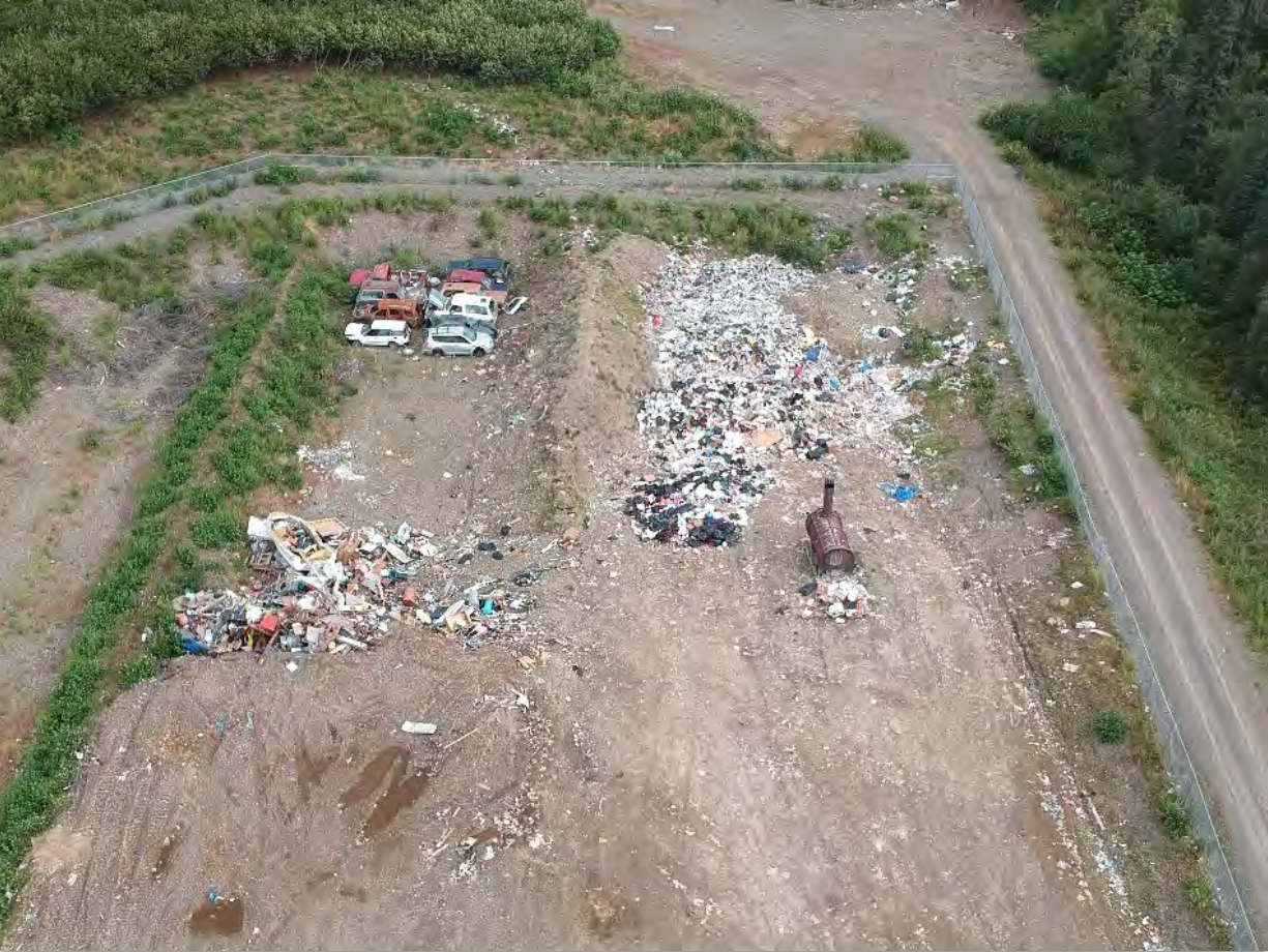
Area fill landfill with the household waste consolidated behind the burn unit. The waste on the left side is construction and demolition debris.
