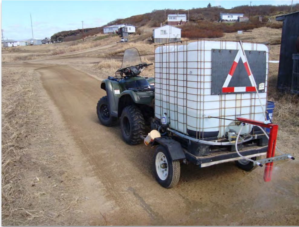
Clean well-maintained equipment used to water the landfill road to help prevent dust.
