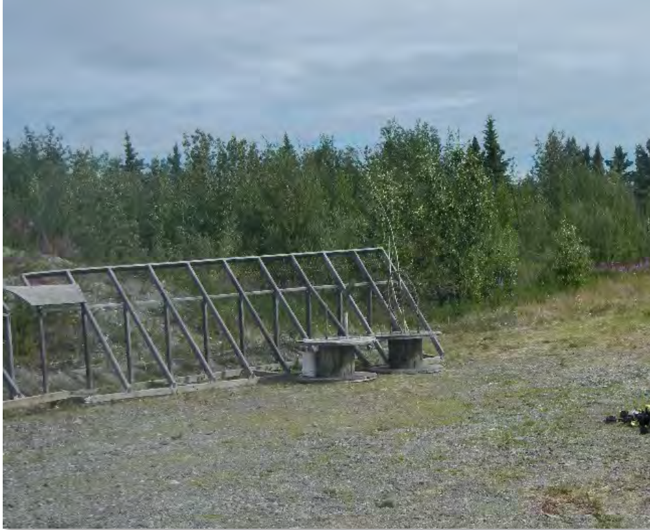
Homemade moveable litter fence near a trench.
