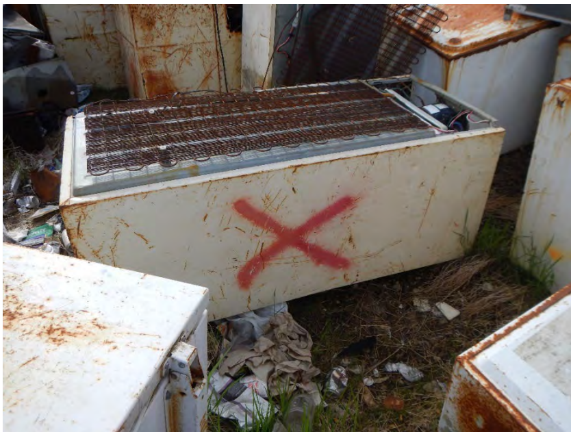
Refrigerator marked after the CFCs have been removed.
