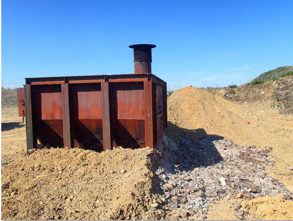
Enclosed commercial burn unit.
