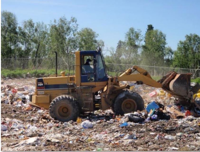
Landfill operator consolidating waste.
