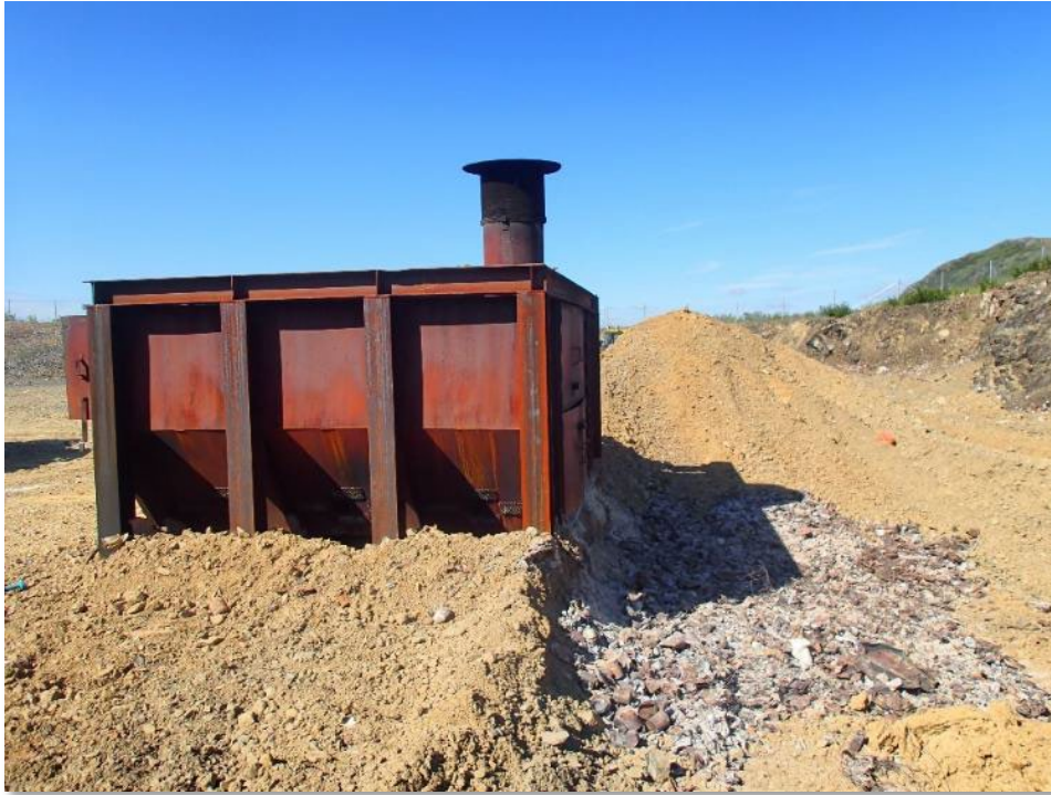
Enclosed commercial burn unit.
