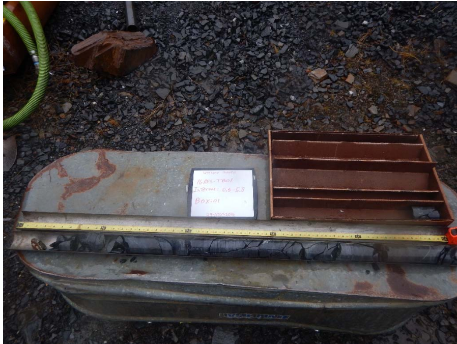
Photo 3: Rock core from 0.8 to 5.8 ft bgs of borehole P-01.
