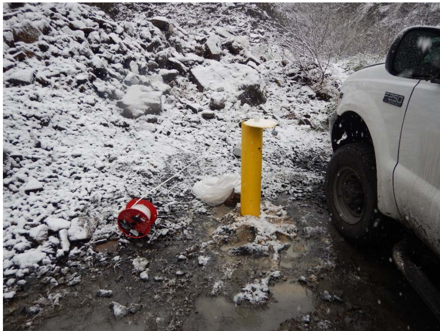
Photo 8: Initial readings of groundwater elevation in P-01 after development of well. Date: 12/3/2016
