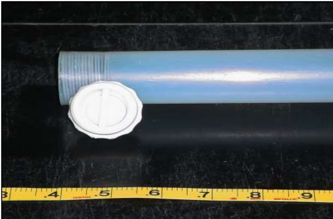
Figure 18. Teflon® constructed bailer with Teflon® ball check valve (Photograph by J. Schoenleber)
