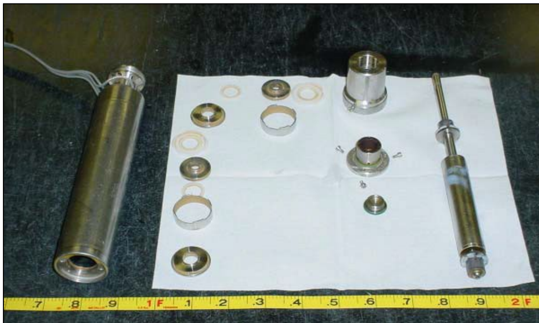
Figure 9. Disassembled Grundfos® Pump being prepared for decontamination (Photograph by J. Schoenleber)
