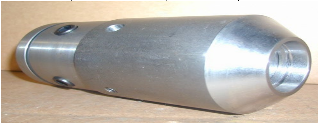
Figure 5. Shelby Tube Sampler (photo taken from Diedrich Drill, Inc.)
