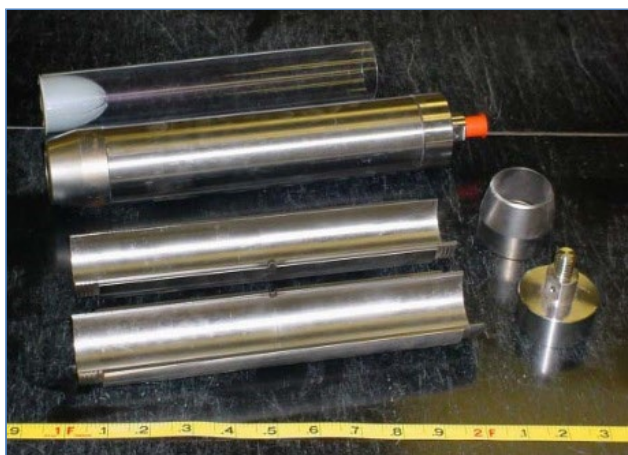
Figure 3. Soil Coring Device (Photograph by J. Schoenleber)
