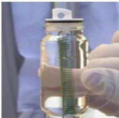
Figure 16. Snap Sampler™ VOA Vial
