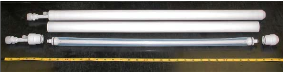
Figure 7. Example of a Teflon® constructed bladder pump, complete (top) and exploded version illustrating internal Teflon® bladder (Photograph by J. Schoenleber)
