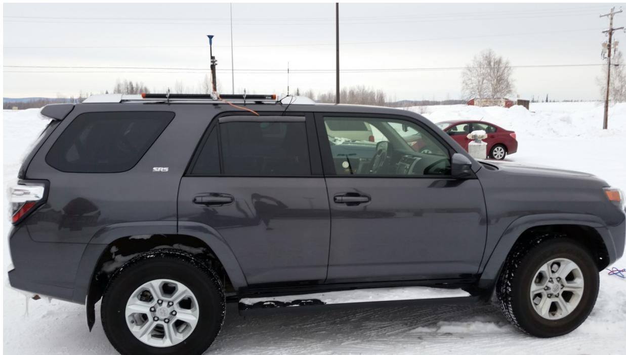
**Figure 3-3: Mobile Sampling Vehicle with Sample Inlet on Top.**
