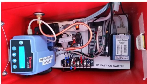
Figure 3-2: Instrument Configuration for the Mobile Monitoring Sample Enclosure.
