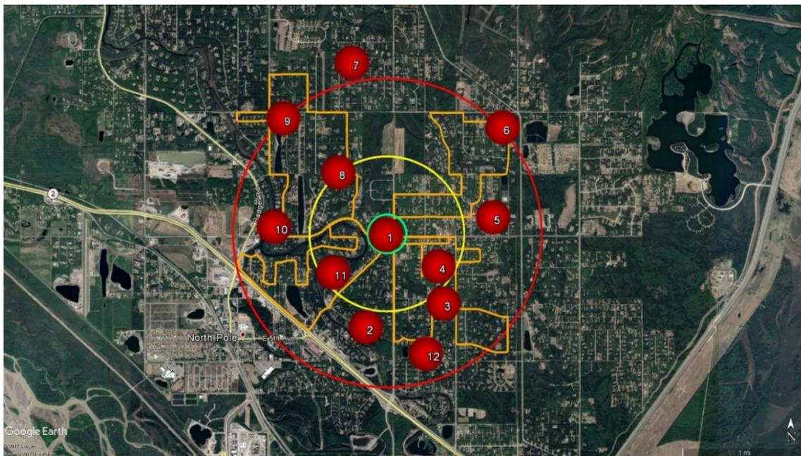
Figure ES-1: North Pole Saturation Study Fixed Monitoring Sites (Large Red Dots) and Mobile Monitoring Routes (Orange Lines).
