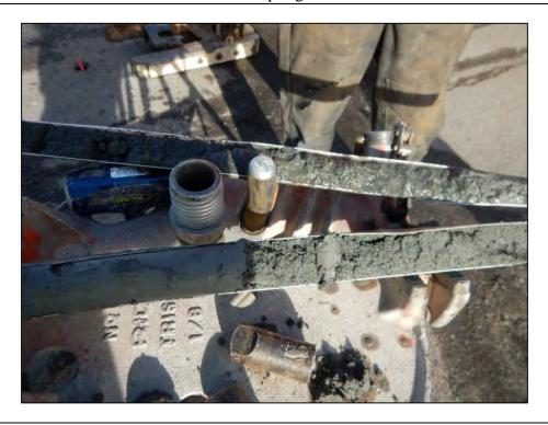
Photograph 8: View of soil core at GW-49. Silt to saturated sand transition visible.
