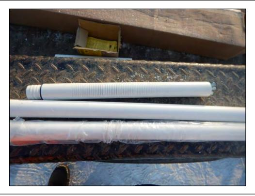
Photograph 2: Vapor monitoring well screen and casing.
