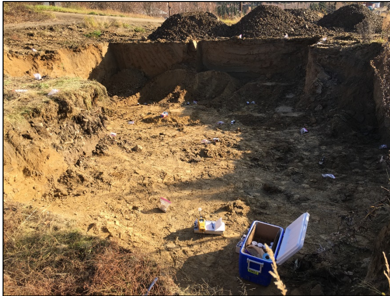
Photo 27. Sampling base of excavation (empty jars staged at sample locations).
