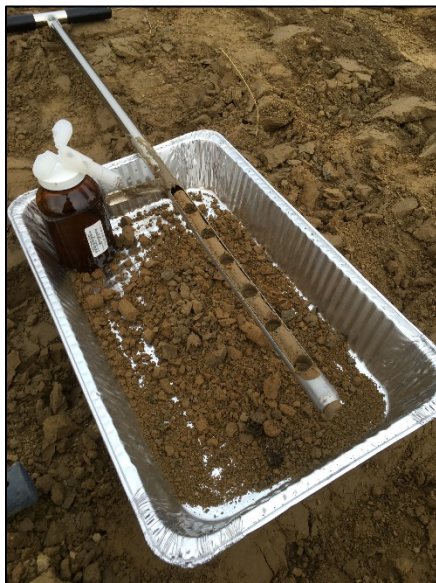
Photo 36. Subsampling ISM core using Terra-core (for GRO/BTEX).
