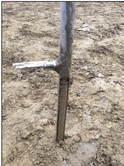
Photo 35. Soil probe used to obtain ISM soil cores (increments).
