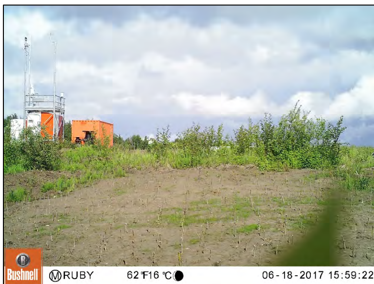
Photo 30. Leaf in foreground (lower right) setting off motion capture every minute
