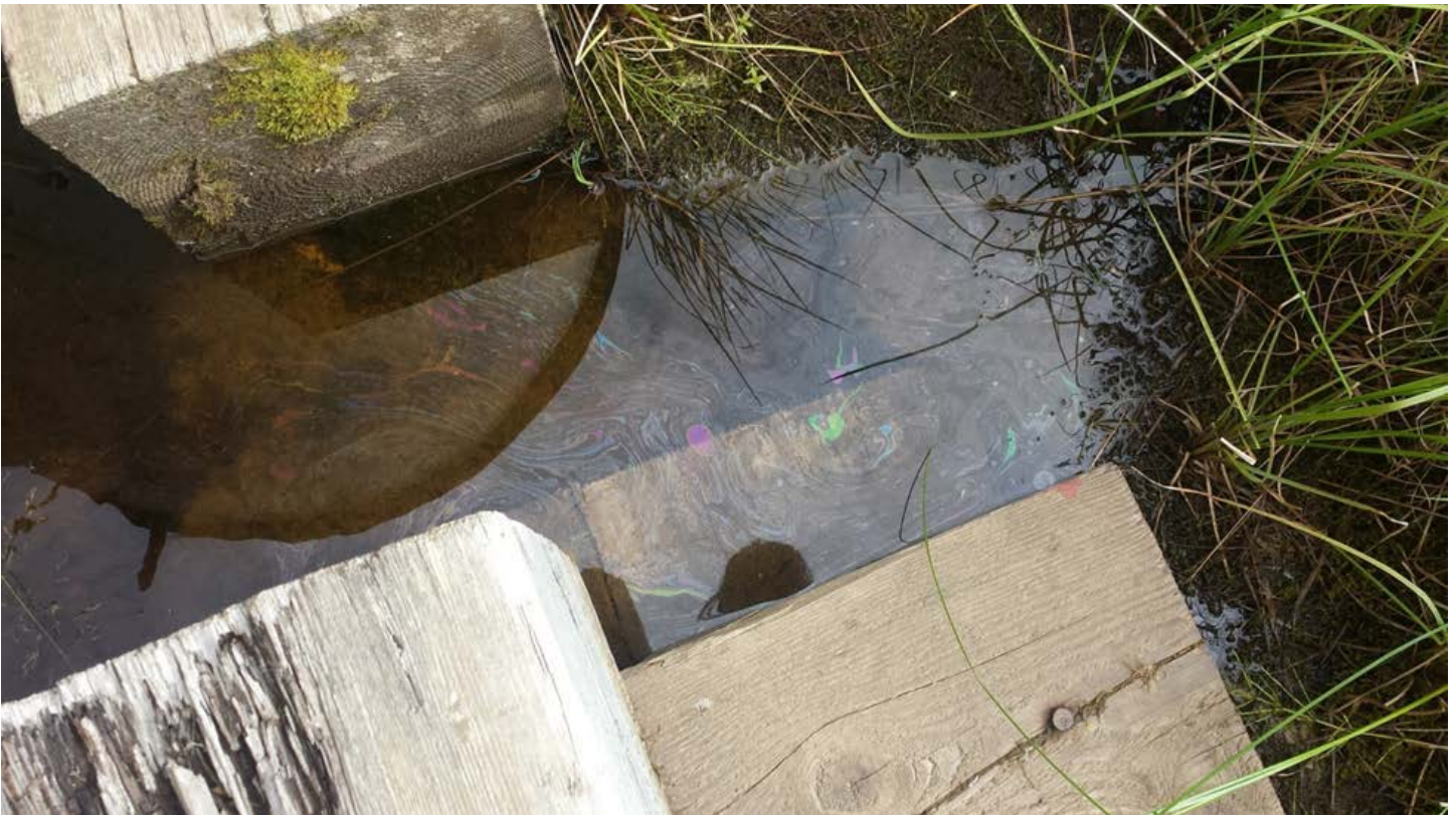
Photograph 10 – Standing water with a sheen found around and under the property's tank farm.
