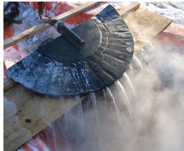
Figure 43. Manta ray skimmer used as inlet hose to prevent erosion
