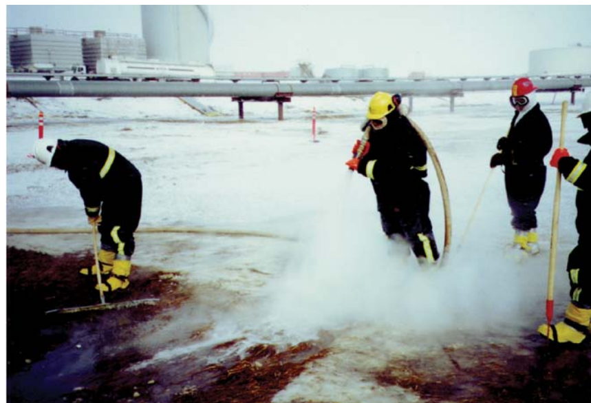
Figure 47. Flushing tundra with surfactants
