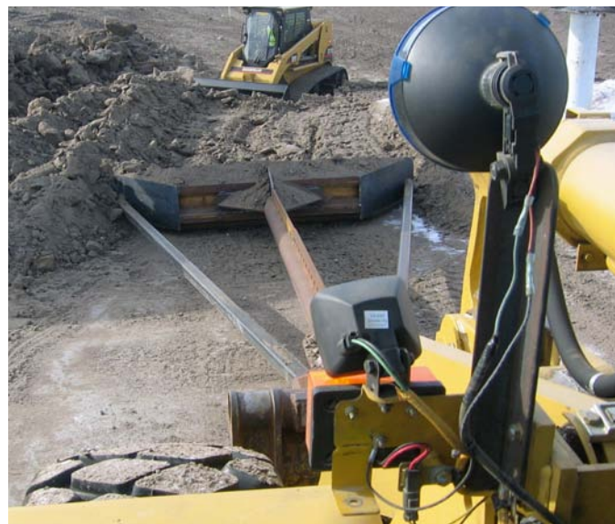
Figure 27. Loader extension pushing material
