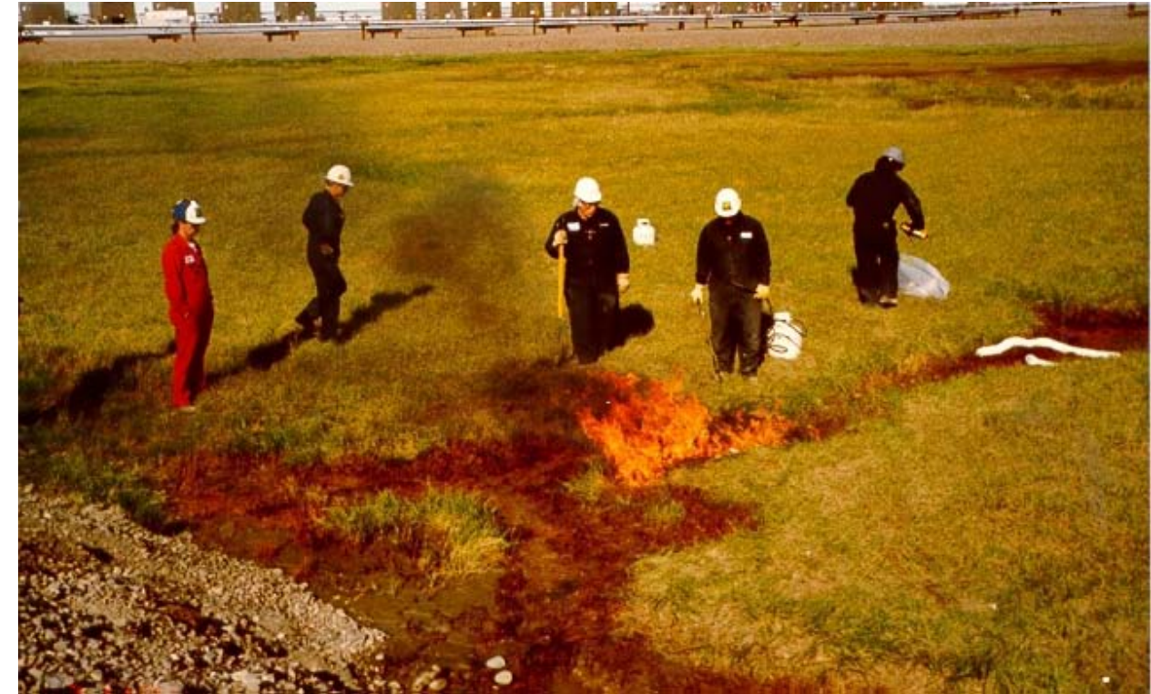
Figure 53. Burning a thin layer of surface contamination
