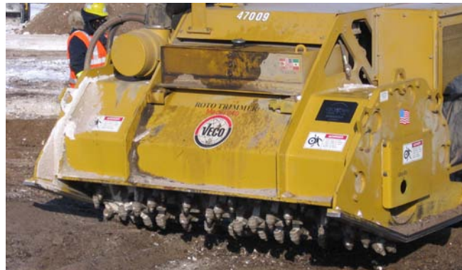
Figure 65. Trimmer excavating contaminated soil
