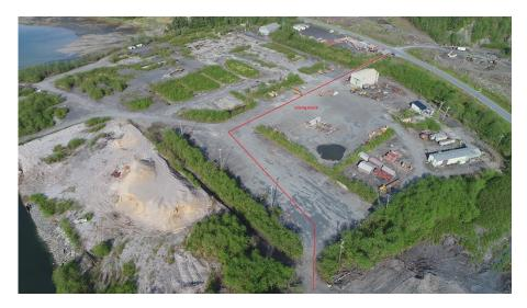
Once all contaminated materials have been containerized and removed from the site. The area under the current stockpile will be sampled to ensure it is free from contamination and then the site will be leveled and closed.
