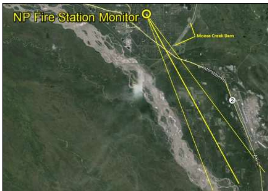
Figure 6-10 Preferred Wind Directions for PM 2.5 Concentrations at FNSB NP Fire Station Monitor at a Bearing of 151°
