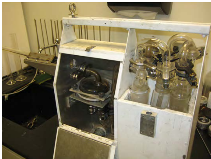
Figure 3. Ammonia Sampling Probe and Impinger Train
