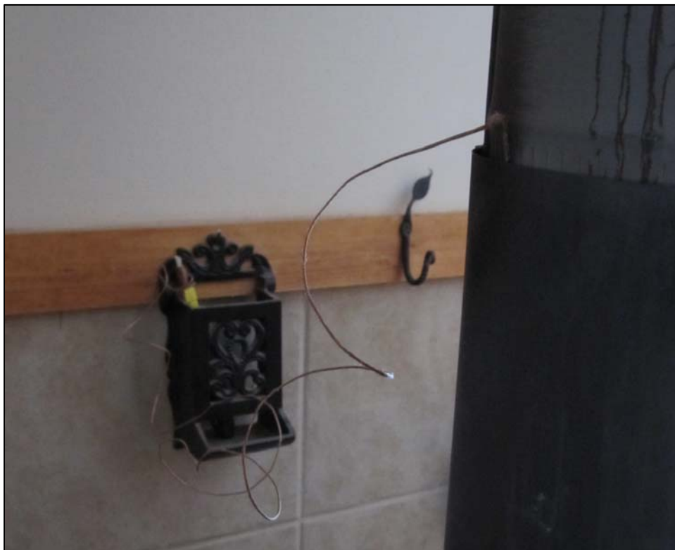
Wood stove flue pipe with a high-temperature thermocouple inserted in the joint between two sections. The thermocouple connects to a datalogger stored in the matchbox holder in the background.
