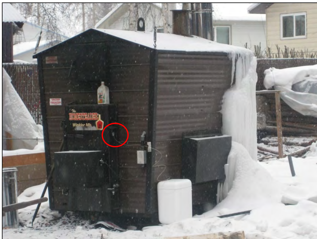
Thermocouple placement for outdoor wood boiler at OWB-2.
