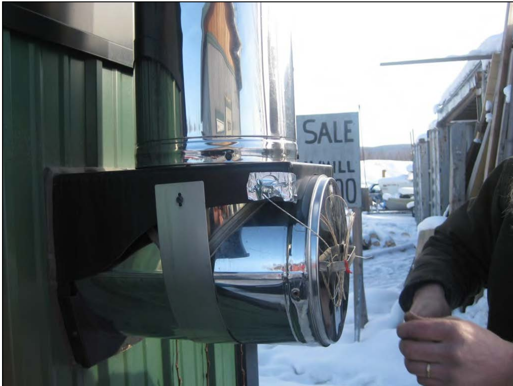
Thermocouple placement for outdoor wood boiler at OWB-1.
