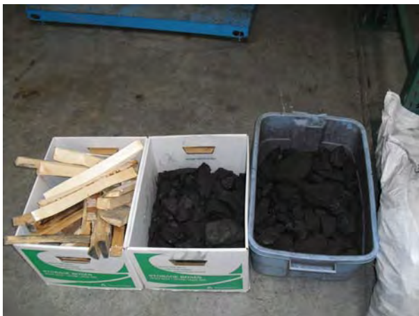
Run 36 (wet lump coal low, cold start) test fuel-kindling, preburn, test fuel
