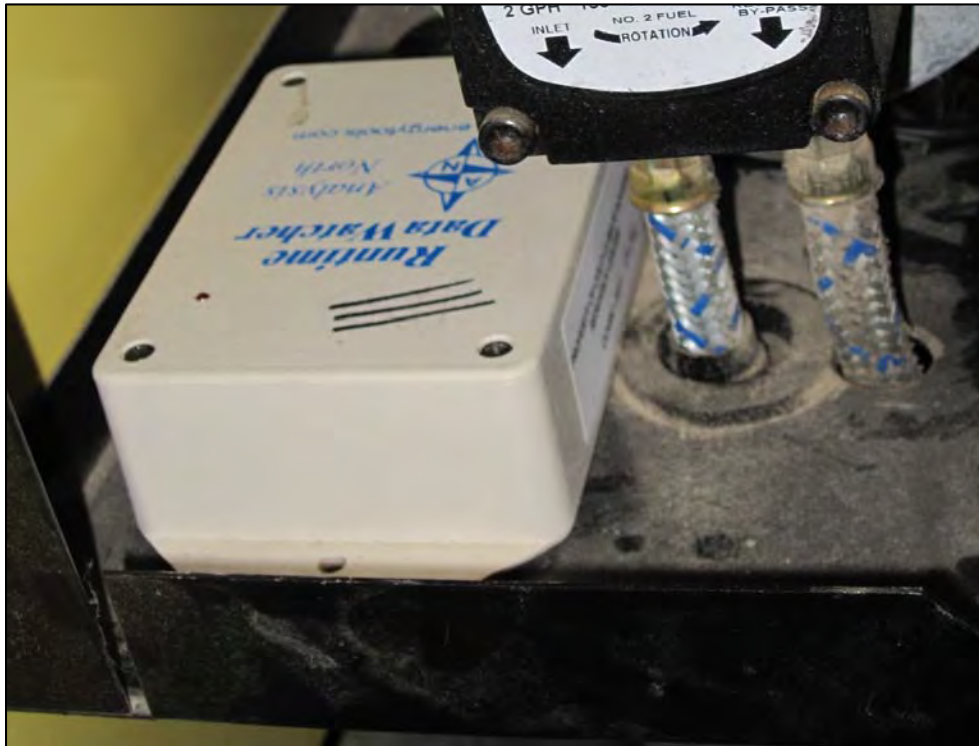
Example of a Runtime DataWatcher datalogger being installed to monitor an oil boiler.
