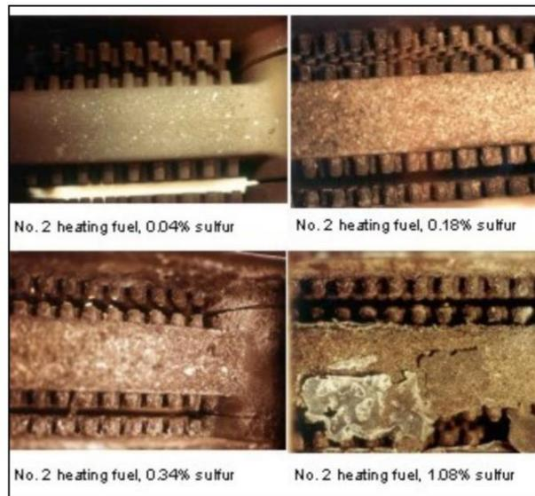
***Figure 9: Buildup of Soot and Particulates on Heat Exchange Plates for Identical Boilers using Different Fuels***
