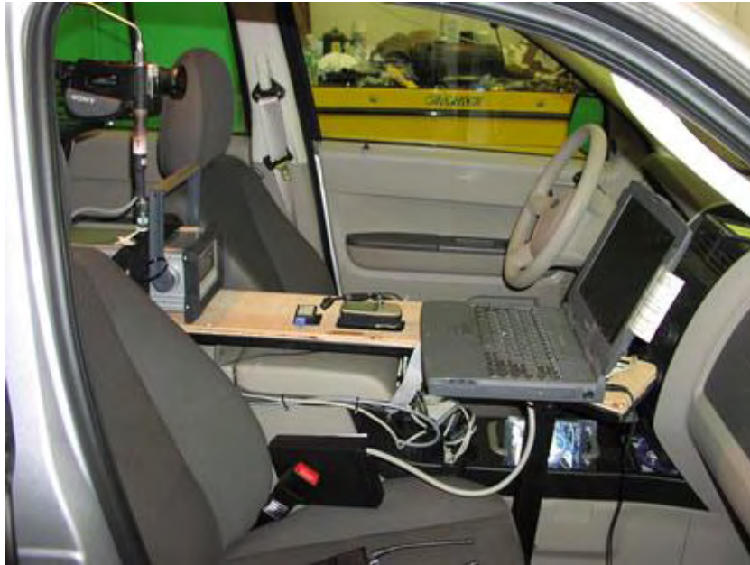
Figure 2-5 Interior of FNSB Vehicle Camcorder, 2 nd of two in-line heaters, DataRAM, GPS, thermocouple datalogger, Toshiba laptop, and Rotary Switchbox (backside)
