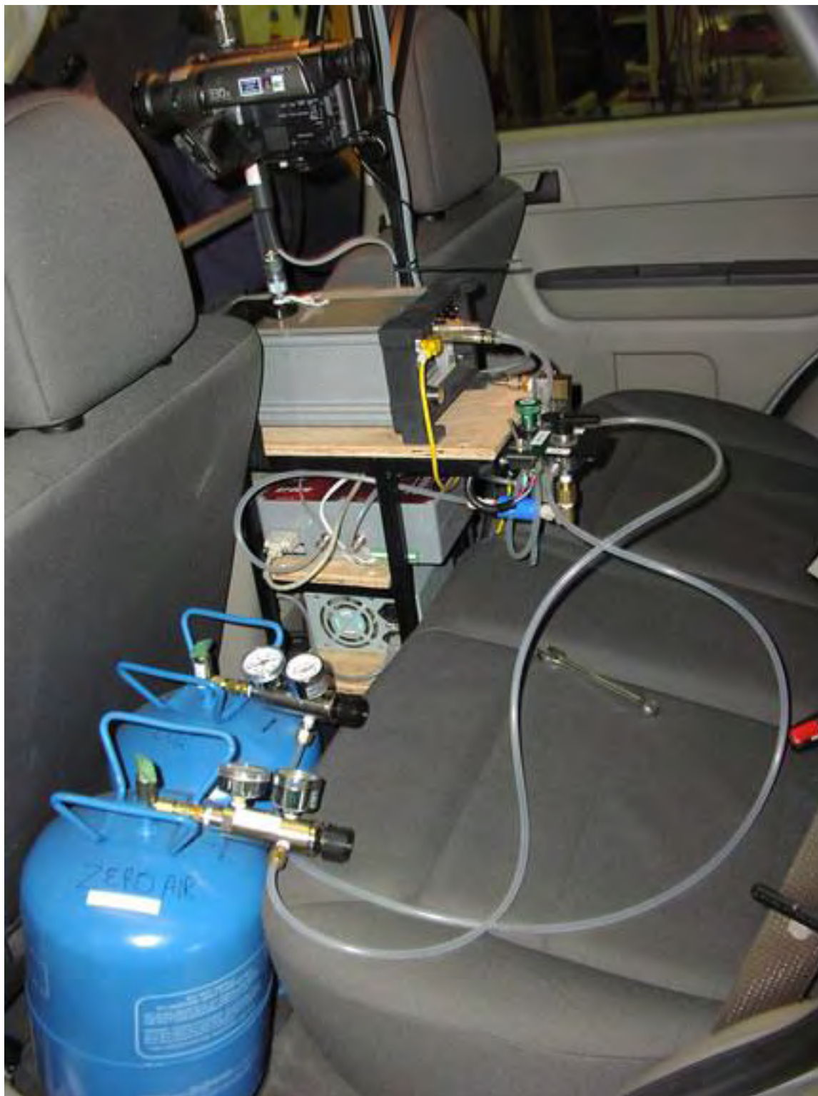
Figure 2-7 Back Seat Area of FNSB Plume-Following Vehicle Camcorder, in-line Heater, DataRAM, LI-COR, Power Supply, and Calibration Gases
