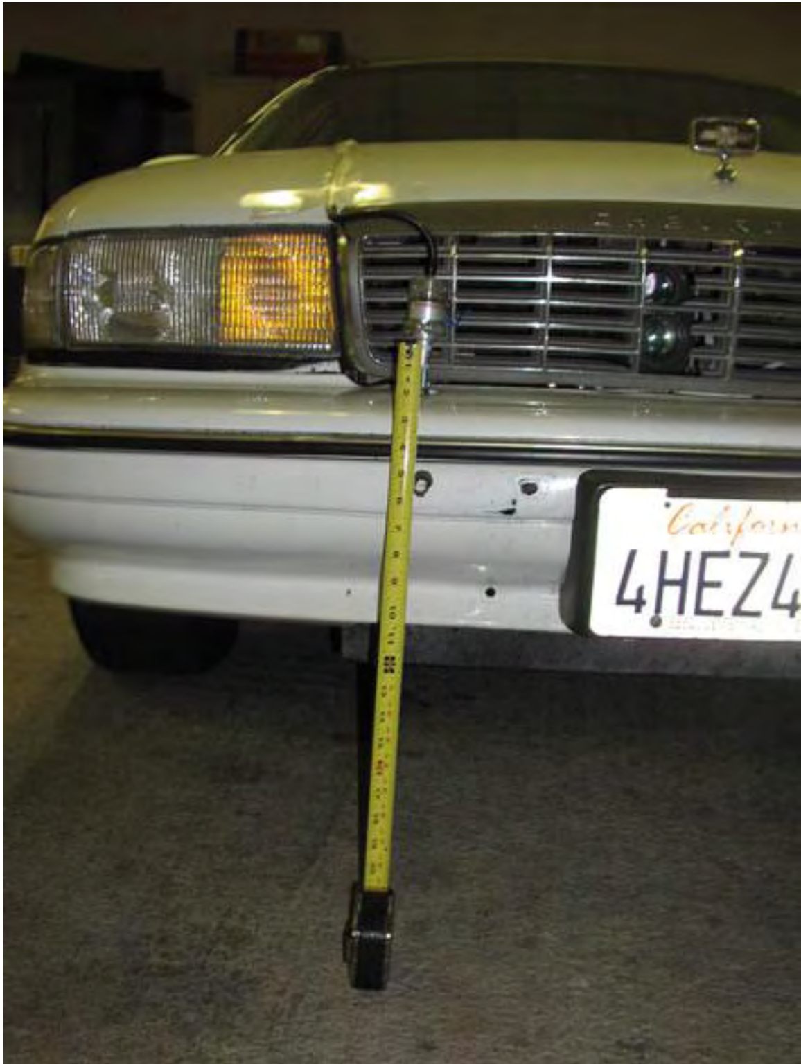
Figure 2-2 Caprice (prototype plume follower) Front Bumper Mount of BGI Cyclone
