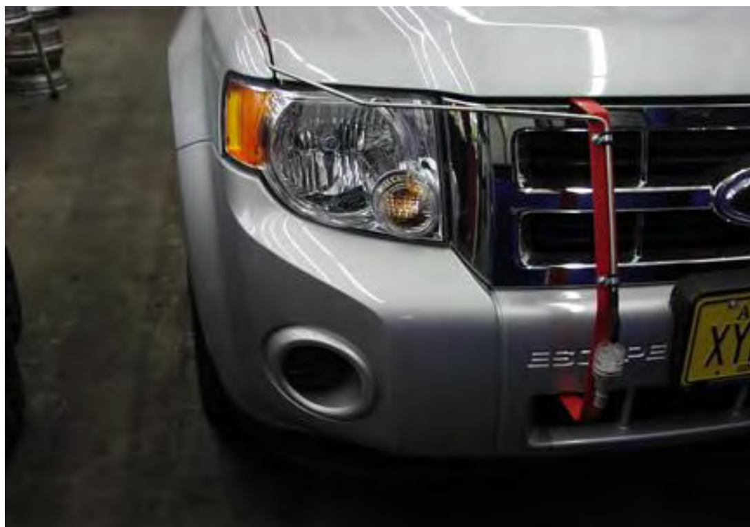
Figure 2-4 Bumper-Mounted Primary Sampling Cyclone on FNSB Plume-Following Vehicle
