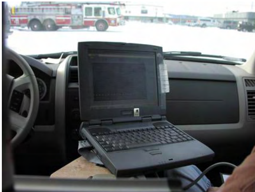
Figure 2-6 Laptop Inside FNSB Plume-Following Vehicle Provided 20-second real time display of CO 2 and PM 2.5 Concentrations (PCMCIA A/D card plugs in at left, attached to ribbon cable)
